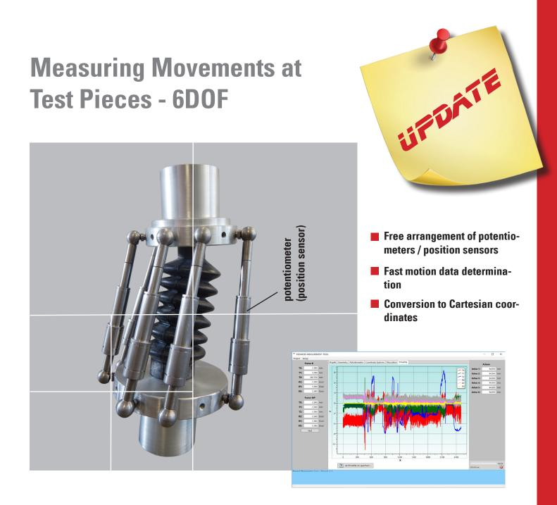
Hexapod-test facilities are perfect to simulate movements in all dimensions and rotation. However, in order to do so, we first need to obtain the respective motion data - and sometimes it can be tricky to measure these movements at test pieces or components. **HexMeas** software helps you to accomplish this task.
