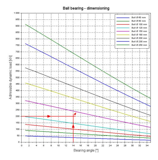
The graphic above shows the possibility of Hagenbuch ball joints. It shows the relationship between the maximum possible bearing angle, the maximum admissible force and the required ball diameter. All possible combinations of force and angle are possible with the standard Hagenbuch construction. Special ball joints can also be developed on request, for example for tight spaces or if the needed tensile and compressive forces are different.
